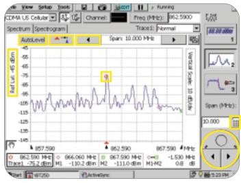
**Figure 5b.** Automatic spectrum features.
