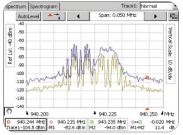
Figure 28c. N-PCS spectrum varies continuously.
