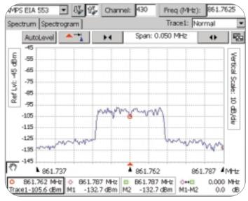
Figure 26. SMR (specialize mobile radio) signal.
