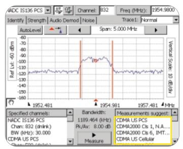
**Figure 4.** Interference identity screen.
