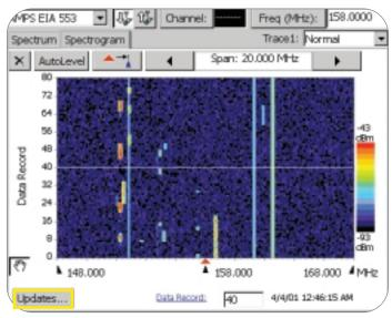
Figure 9. Completed spectrogram.
