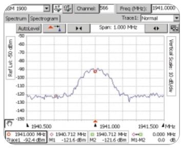
Figure 21. A GSM cellular signal.
