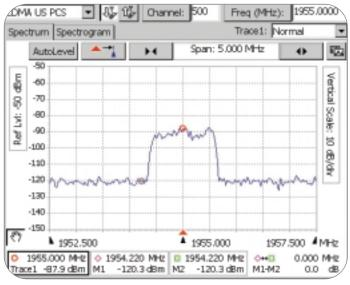
Figure 22. CDMAOne (using 5 MHz span).
