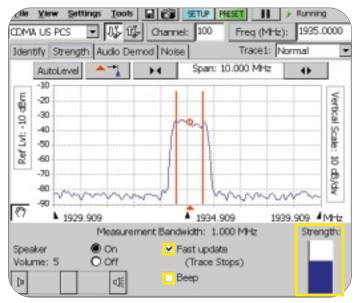
Figure 14. Measuring interference strength.
