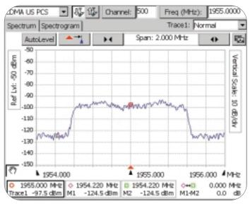
Figure 23. CDMAOne (using 2 MHz span).
