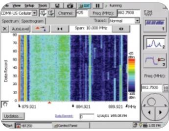
Figure 10. Spectrogram of live cellular signals.
