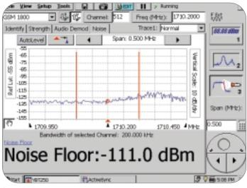
Figure 3b. Higher noise floor due to interference.
